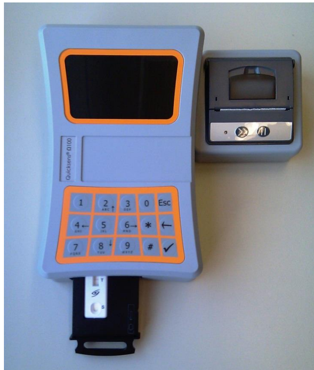
Figure 2: Reader QuickSens® Ω100 with printer attached and with test inside slide-in module
